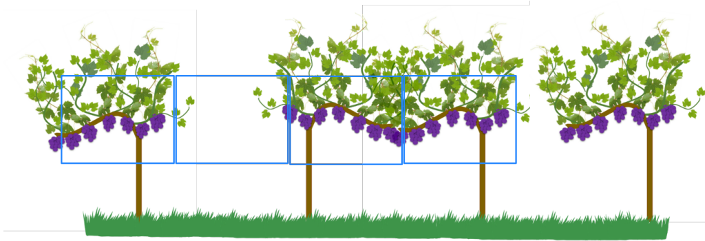
Figure 7: Image selection based on the geo-referenced image coordinates with the goal of minimal overlap between selected images.
